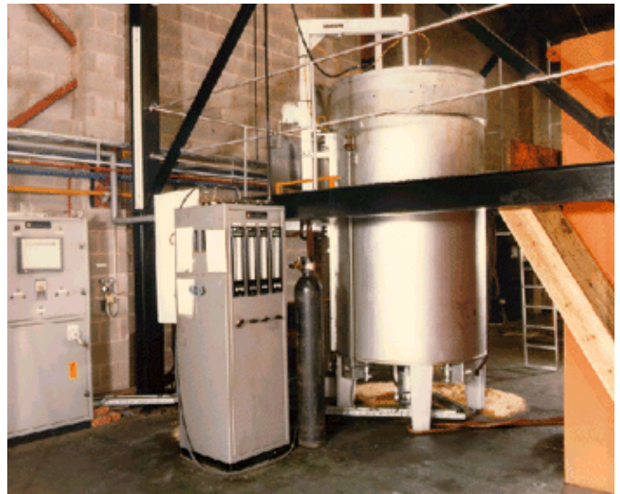
Figure 4. A pit furnace for nitriding and nitrocarburising
