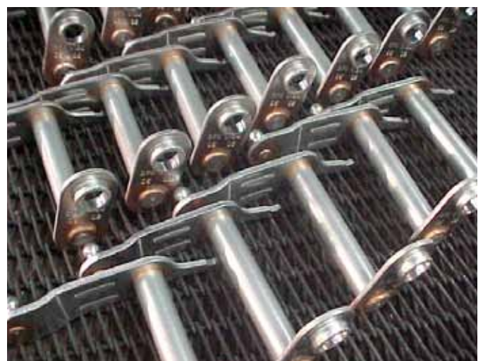
Figure 2. Copper brazed mild steel select lever assembly
