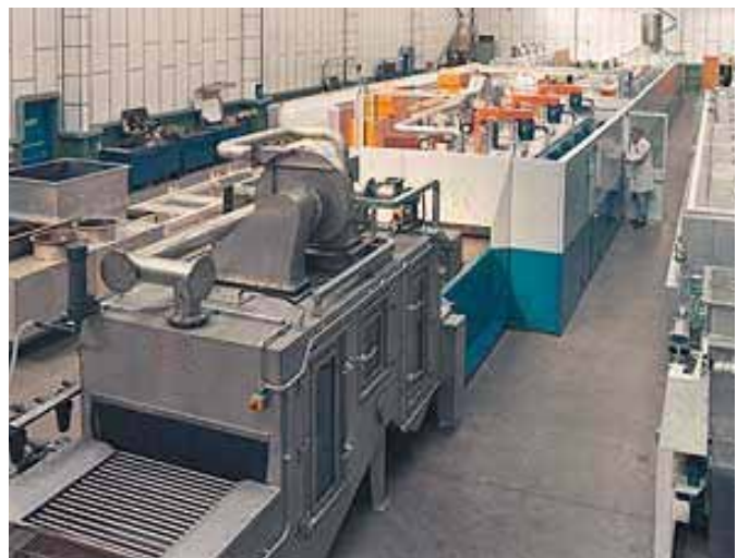
Figure 5. A typical aluminium brazing furnace
